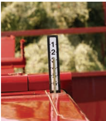
Distance Indicator is easily visible from the tractor seat. It shows you the relative distance bales are thrown: six is the farthest distance (fastest belt speed); one is shortest.
