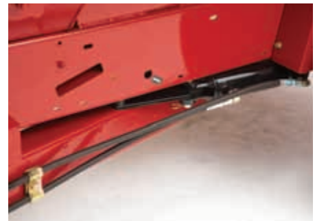
Hydraulic tongue swing uses hydraulic muscle to swing the baler into transport or working position quickly and easily.
