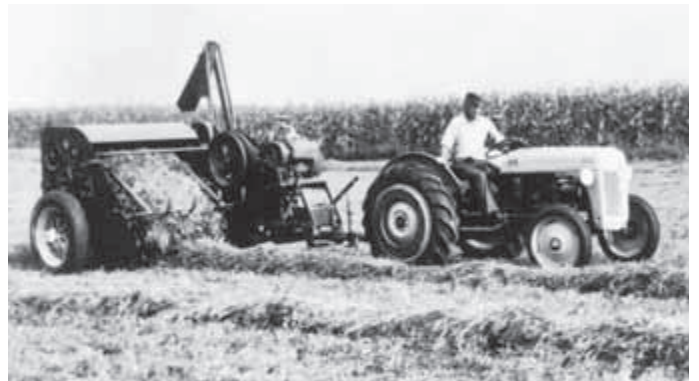
Ed Nolt, inventor of the first successful automatic baler, field tests an engineering prototype in the mid-1940s. His design revolutionized hay and straw harvesting and earned New Holland a place of honor in the history of agricultural machinery.
