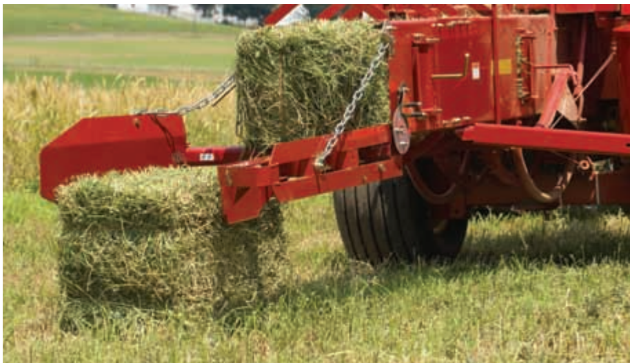
Quarter-turn bale chute drops bales on their sides so twine is kept away from the ground to prevent rotting. Sets bale into proper position for retrieval by automatic bale wagon. Bale case extension is also recommended when using the quarter-turn bale chute.
