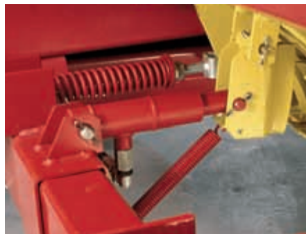
Hydraulic pickup lift. (Shown from rear of baler.) When baling, raise or lower your pickup as needed to adjust to differing terrain without leaving your tractor seat.
