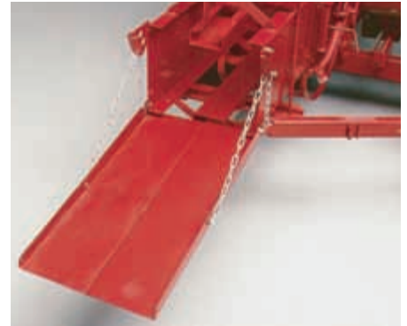
Triple-purpose chute supports bales as they leave the chamber; can be set to roll bales to the left, away from the next windrow. (Also becomes the base for bale-loading chute.)
