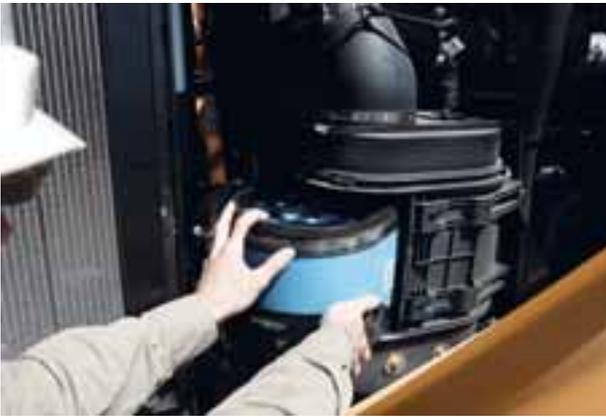
The air filter is easy to remove and the dust is aspirated and ejected in the exhaust
