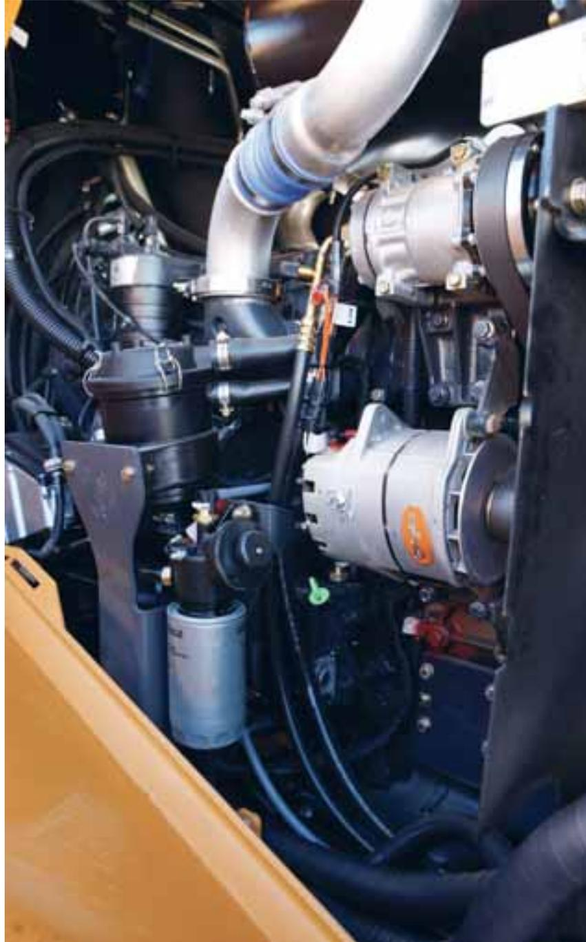
Fuel filter and engine oil service points are easily accessible from the left side while the other filters are behind the right stairs
