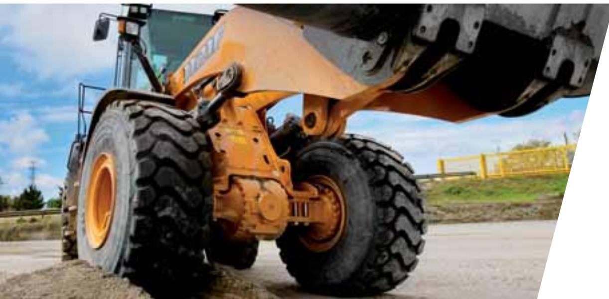
For a reduced initial investment, the axles are also available with both open differentials without locking. In that configuration the front axle is heavy duty and the rear axle is standard.
