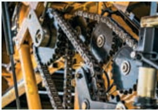
Stronger driveline - new gearbox and drive chains.
