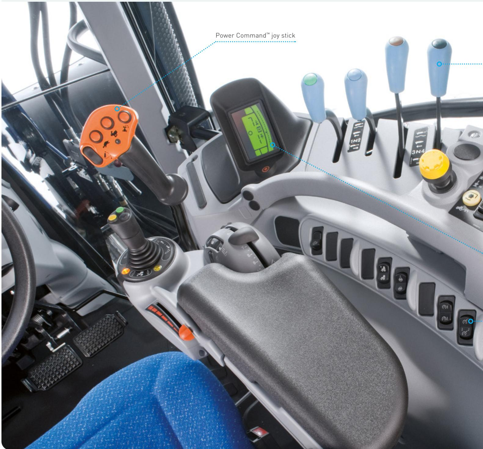
With the Classic armrest, you enjoy easy access to mechanical remote levers, PTO engagement, switches to control 4WD engagement, differential lock, auto shift range function, and more. You can also easily perform quick, clutch-free gear changes with the Power Command™ joystick.
