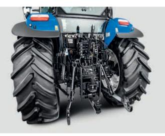
Equip a New Holland T5 with front linkage and PTO, and you have a tractor that's even more versatile. The new wet-clutch PTO design is maintenance-free and ensures quieter operation.
