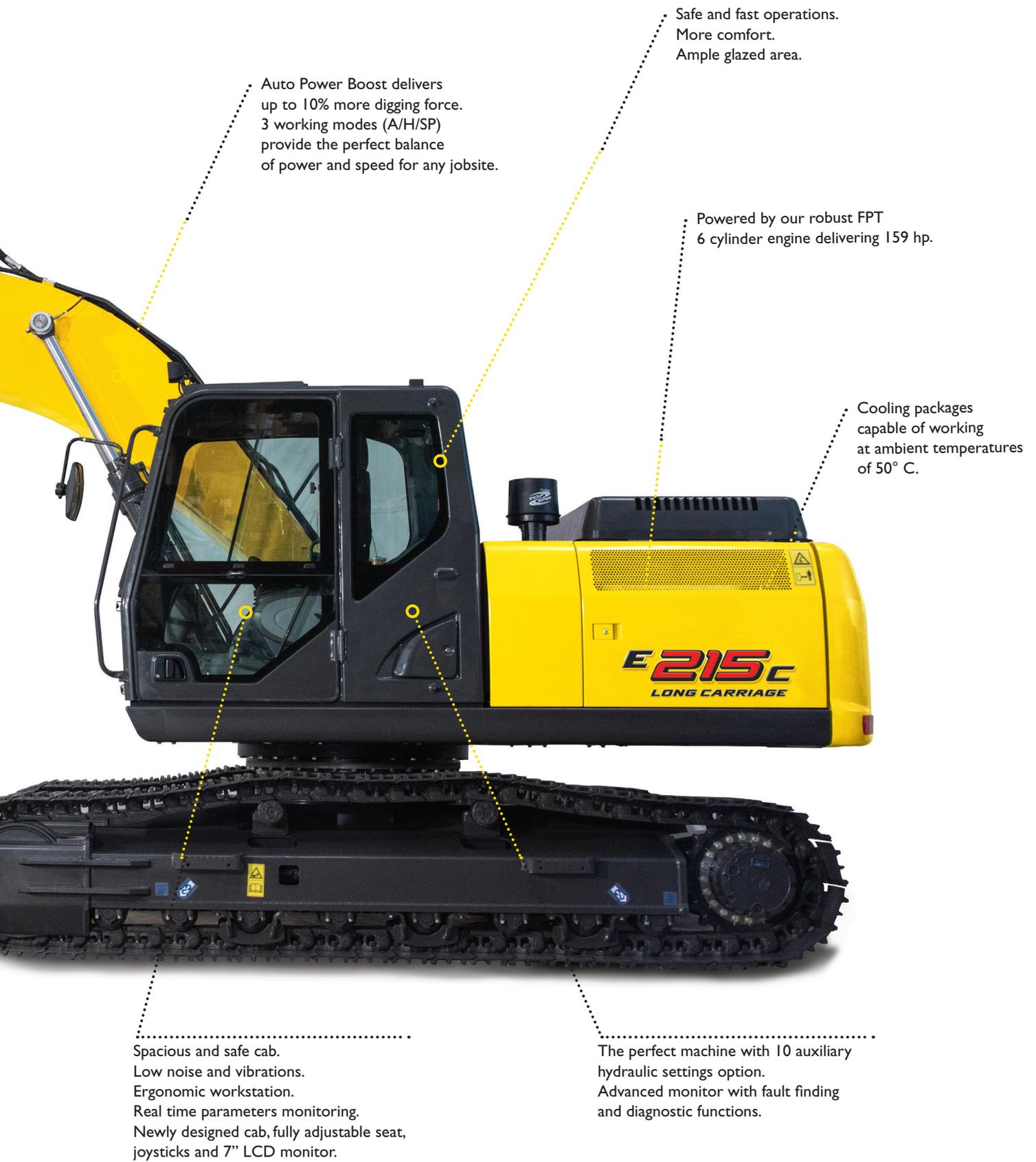
Auto Power Boost delivers up to 10% more digging force. 3 working modes (A/H/SP) provide the perfect balance of power and speed for any jobsite.
