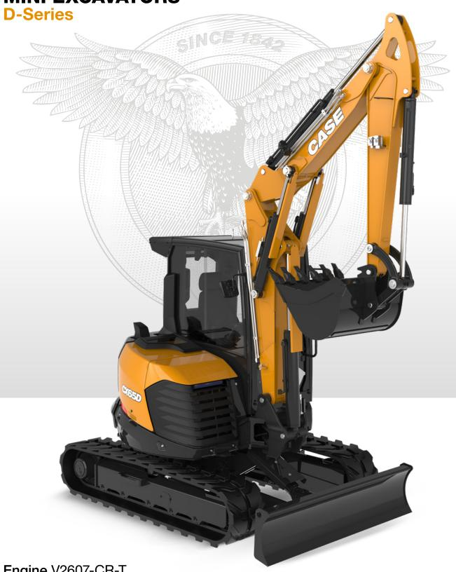
Engine V2607-CR-T Engine power 44.3 kW - 59.4 hp Operating weight 6520 kg
