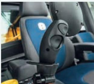
Shift button and ground speed unlock (behind)
