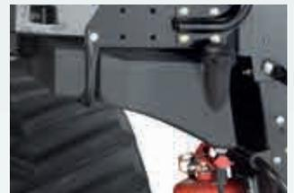
The integrated water tank is placed ideally for washing hands before cab entry.
