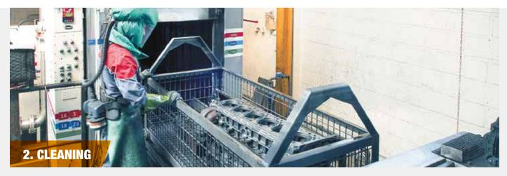
Each component is thoroughly cleaned and verified following the latest original new parts specifications.
