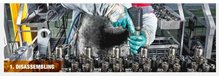
All cores are completely disassembled for inspection.
