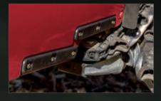
**Replaceable wear strips** are easy to service, keeping you in the field during optimal harvest windows.
