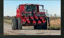
Case IH offers folding corn heads in 8-row and 12-row configurations. Capable of **folding into transport mode in less than a minute,** folding heads dramatically improving transport efficiency, and, ultimately, field productivity.
