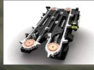
A large, open **front-gathering chain sprocket** sweeps stalks efficiently into rolls and helps harvest downed cornstalks.
