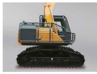
Strong and stable to operate on the soft underfoot conditions, i.e peat land with 7 ton payload. Standard track shoes 960mm Single Grouser, 171kN tractive effort. 580mm ground clearance
