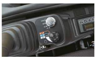
Operators can store up to 10 auxiliary hydraulic flow hydraulic flow and pressure settings to easily switch among different attachments with no need of any mechanical adjustment.
