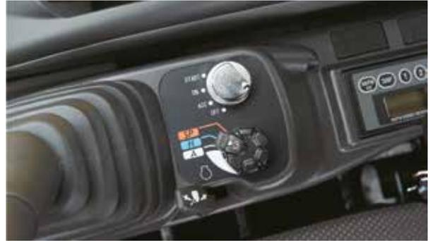
Operators can store up to 10 auxiliary hydraulic flow and pressure settings to easily switch among different attachments with no need of any mechanical adjustment.
