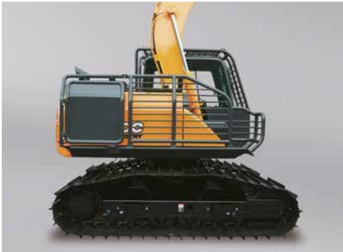
Strong and stable to operate on the soft underfoot conditions, i.e peat land with 7 ton payload. Standard track shoes 960mm Single Grouser, 171kN tractive effort. 580mm ground clearance
