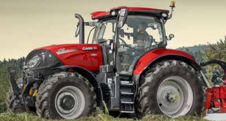
The 6.7 litre 4-valve engine with Common Rail high-pressure fuel injection and wastegate turbocharger delivers performance, torque, fuel efficiency and reliability between 140 and 180 hp (rated). All models benefit from an Engine Power Management boost for PTO, hydraulic and transport work, taking those figures to 175 to 225 hp.
