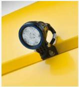
Rear lamps enable operators to monitor residue and two lamps located on the side panel illuminate the rear axle to prevent crushing standing crop and to assist when manoeuvring
