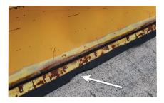
REPLACE ONLY DAMAGED SECTION Should a cutting edge become damaged, simply replace the section instead of replacing the entire length of a costly steel or rubber cutting edge. In the unlikely event of major damage to a section, it can be easily removed and replaced with a new replacement part from your CASE dealer. With conventional snow pushers, major damage usually results in a total loss.
