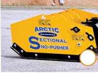
For wear shoes to lay flat on the pavement, other snow pushers with fixed side panels and rigid mounting systems are difficult and time-consuming for an operator to adjust. With this forward-thinking sectional design, wear shoes always lay flat. Made of Hardox 450 hardened steel, the shoes will last through several winters of commercial use.
