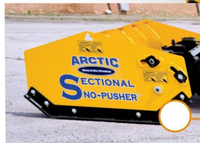
For wear shoes to lay flat on the pavement, other snow pushers with fixed side panels and rigid mounting systems are difficult and time-consuming for an operator to adjust. With this forward-thinking sectional design, wear shoes always lay flat. Made of Hardox 450 hardened steel, the shoes will last through several winters of commercial use.
