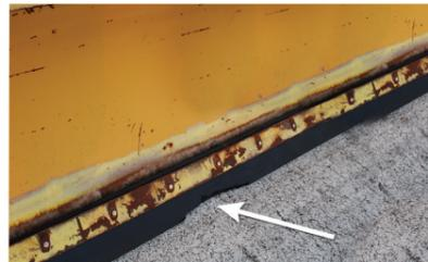
Should a cutting edge become damaged, simply replace the section instead of replacing the entire length of a costly steel or rubber cutting edge. In the unlikely event of major damage to a section, it can be easily removed and replaced with a new replacement part from your CASE dealer. With conventional snow pushers, major damage usually results in a total loss.
