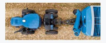
Grain cart applications with VF dual tyres (Row Crop Frame shown) allow for high-speed, low-pressure inflation, which lessens soil compaction while boosting fuel economy. Through less compaction, the T9 Series tractor improves your harvest and yields the following year.
