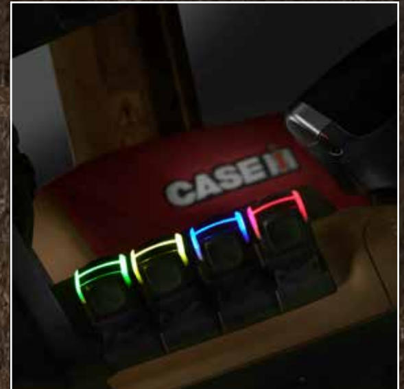
CONFIGURABLE CONTROL SWITCHES ON THE ARMREST WITH CHANGING COLOURS ENABLE THE INDIVIDUAL ASSIGNMENT OF THE REAR CONTROL UNITS
