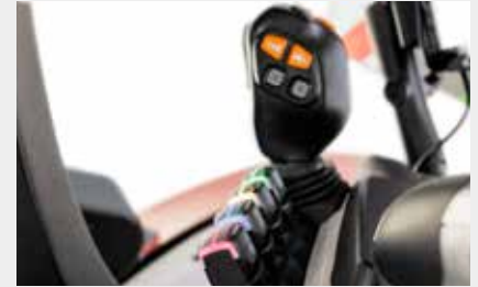
THE JOYSTICK OFFERS PRECISE FINGERTIP CONTROL OF BOTH FRONT AND REAR HITCH FUNCTIONS – FOR SMOOTHER OPERATION.
