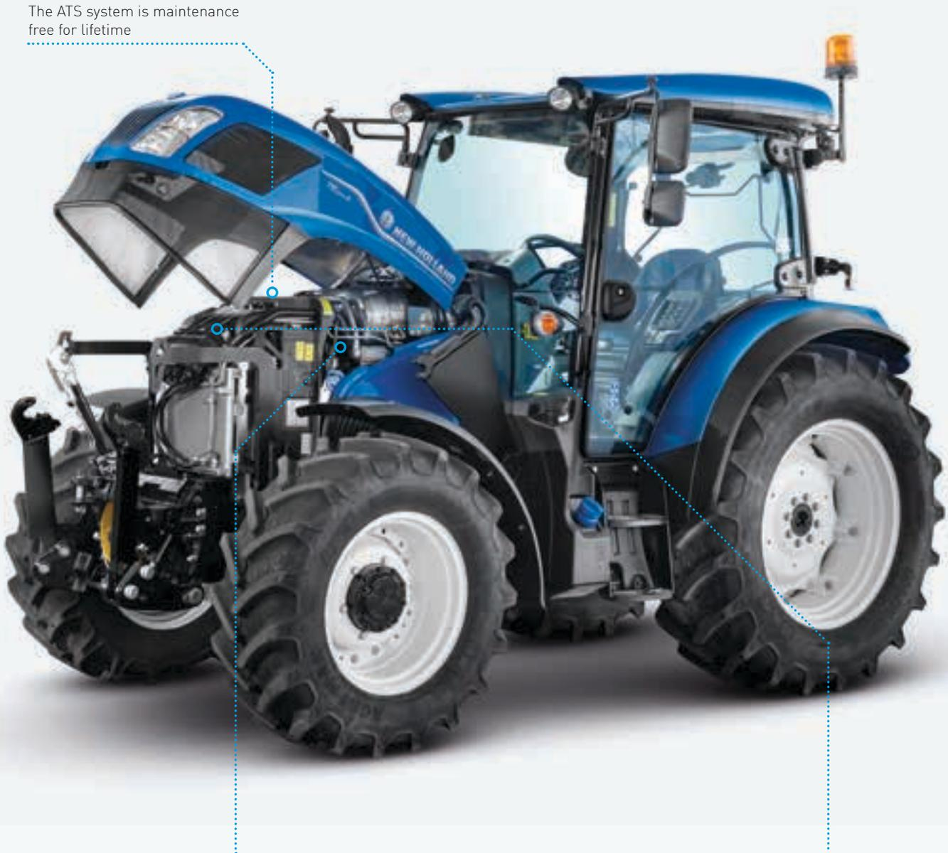
All the maintenance can be done on one side, all service points are on the left side of the engine to make routine servicing easier
