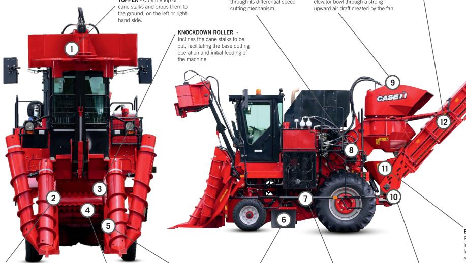
**CROP DIVIDERS** - Two pairs of crop dividers are included to enable separation of the sugarcane row that is being harvested from the adjacent row and lifts the lodged cane stalks to facilitate the feeding operation.
