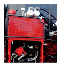
Wire mesh railing on hydraulic tank for additional safety
