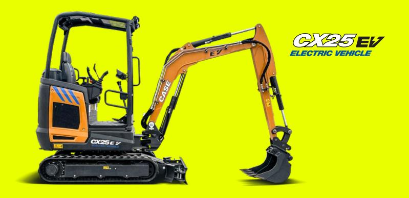
The electric powertrain on the CASE CX25EV mini excavator gives you 25 kW of power and lets you go up to 8 hours on a charge. So, you've got plenty of clean, quiet electric muscle on tap. You also get a full load of features and a choice of canopy or optional cab.
