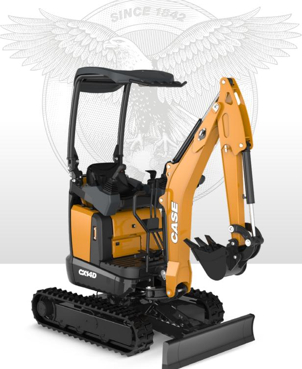
Engine D722 Engine power 8.8 kW - 11.8 hp Operating weight 1360 kg
