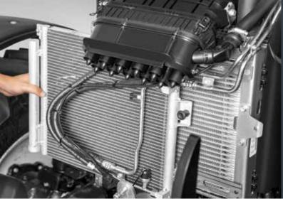
Fast and simple cleaning of the radiator and air-conditioning system.
