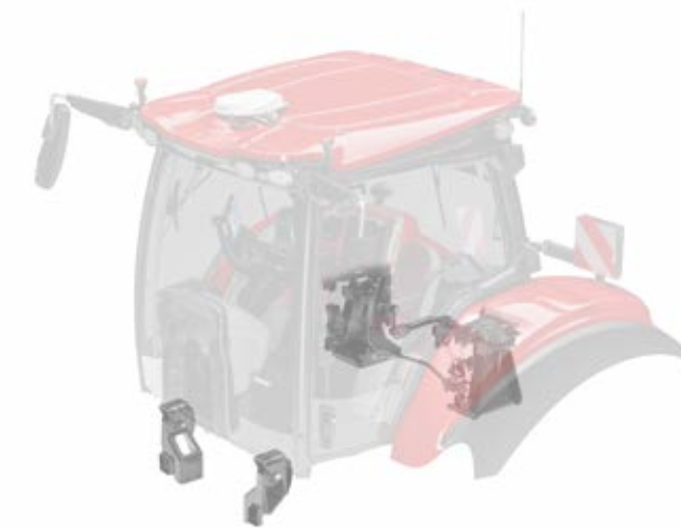
THE SEMI-ACTIVE, HYDRAULIC CAB SUSPENSION RELIABLY ABSORBS JOLTING AND VIBRATIONS.
