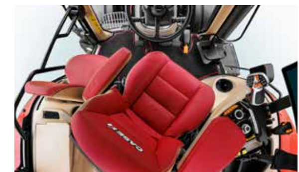
THE SWIVEL SEAT TURNS UP TO 40° – GIVING A CLEAR VIEW OF REAR IMPLEMENTS AND GREATER COMFORT DURING LONG WORKING HOURS.
