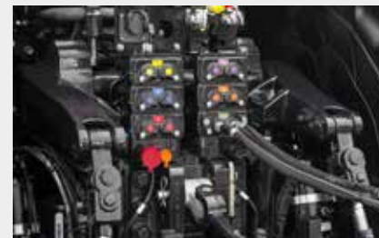
NEW ELECTROHYDRAULIC REMOTE VALVES DELIVER HIGHER FLOW AND FASTER RESPONSE WITH ENHANCED DURABILITY.
