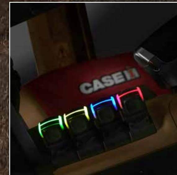
CONFIGURABLE CONTROL SWITCHES ON THE ARMREST WITH CHANGING COLOURS ENABLE THE INDIVIDUAL ASSIGNMENT OF THE REAR CONTROL UNITS
