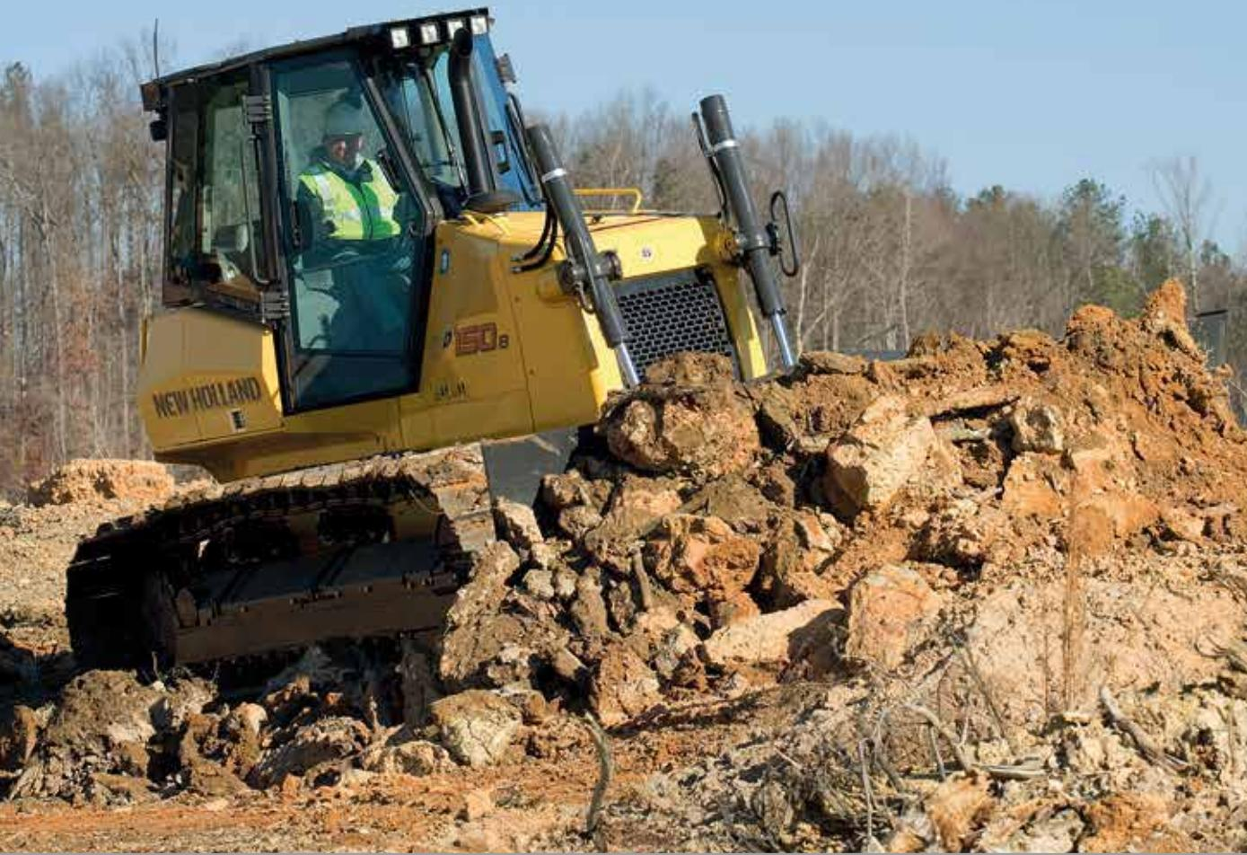
POTÊNCIA LÍQUIDA DO MOTOR 143 hp @ 2.200 rpm
