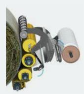
The net knife cuts upward, leaving a clean-cut end.
