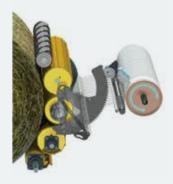
2 Net wrap is applied to the bale when the duckbill pivots into the chamber.
