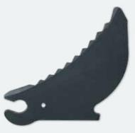
To help lower operating costs, knives can be resharpened, then reused. When cutting is not required, the provided knife blanks can be inserted in the floor. Knife removal is easy. With the tailgate open and locked, unlock the raised knives and simply lift them out. Knife blanks and knives are neatly stowed on the baler.
