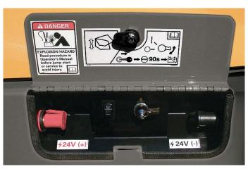
Hood opening and battery on/off switches. In case of flat battery, hood can be opened externally with Remote jump start
