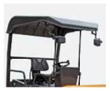
WEATHER PROTECTION CANOPY Large sunroof for protection of the operator from sun and
