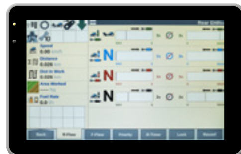
AT-A-GLANCE OVERVIEW OF FLOWRATE AND TIMER SETTINGS ON THE AFS PRO 700™ PLUS MONITOR.
