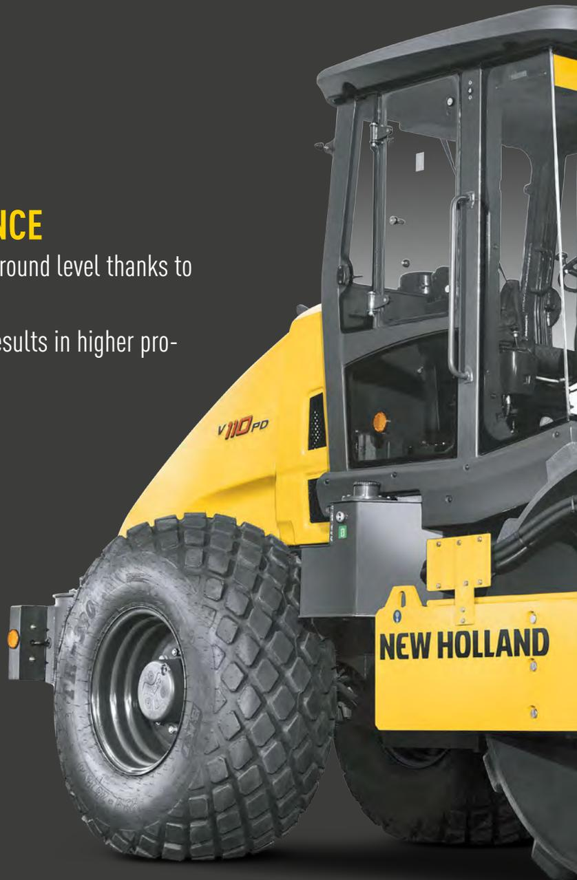
The centrifugal force is generated by an internal eccentric shaft and a rotating mass: depending on the direction of rotation, the rotating mass is either in phase with the eccentric shaft for maximum centrifugal force, or in opposite position, for minimum centrifugal force.
