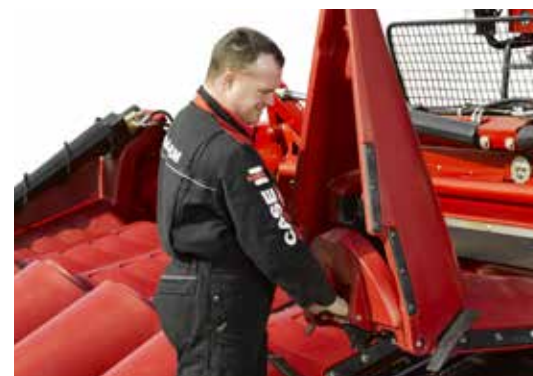
Get access to the row unit by simply lift up the front divider with one hand
