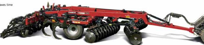
Disk gangs feature spools between the Earth Metal blades, which add weight to increase cutting pressure and clearance for residue flow through the gangs. Four working widths are available to match a wide range of tractor horsepower from larger mechanical front-wheel-drive tractors to the largest wheel or tracked tractors.
