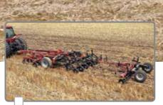
.....The Case IH crumbler combines with the Ecolo Tiger to complete all of your secondary tillage in one pass.
