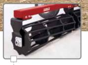
Large 410 mm (16 in.) rigidly mounted reels with heavy-duty bearings (shown with Round rods).
