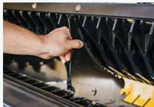
New rotor scraper for improved crop flow and less power consumption.
