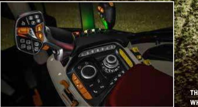
THE ICONS ON ALL SWITCHES ARE BACKLIT WHEN THE HEADLIGHTS ARE ON.
