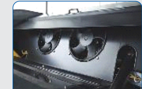
Maintenance Free Knotter Fan-Eliminates Debris Formation
