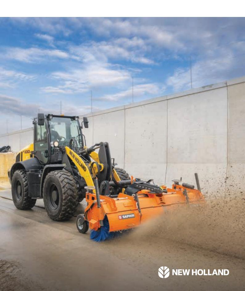
With New Holland hydrostatic drive, you get full pushing power in low gear and maximum speed in high gear. Maximum speed is 40kph, with optional 20kph limiter. Gear transitions are seamless, with no to stop the machine to change gear, providing the best machine efficiency. The W100D also features cruise control option to increase the operator's comfort and 'Eco' mode for reduced fuel consumption, making a significant contribution to low total cost of ownership.
