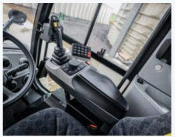
To ensure an ergonomic, intuitive and comfortable environment for the driver, controls have been grouped strategically within easy reach of the multifunction joystick, integrated into the right armrest. For maximum comfort, the armrest is mounted on the air-suspended driver's seat, moving seamlessly with it, even on uneven terrain.
