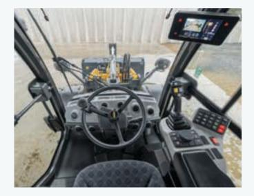
The newly-designed W100D cab offers almost unobstructed 360° vision. An elevated driving position and the abundance of glass surface within four narrow pillars ensure the best possible view in every direction. Access is easy and straightforward via the wide-opening glass doors, and operators will appreciate the bright, airy space and low noise levels of 71dB(A).
