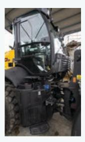
The spacious ROPS/FOPS Level 2 certified cab integrated into the W100D design features fully-glazed doors both on the left and the right, providing easy access and an unobstructed allround view when manoeuvring, maximising both safety and operating efficiency. Grab handles have been placed exactly where you need them, to ensure safe entry and exit.
