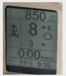
PUMA MULTICONTROLLER MODELS: THE RANGE AND GEAR SELECTIONS ARE CLEARLY SHOWN ON THE A-PILLAR DISPLAY
