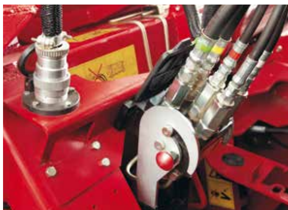
Mount the header in a matter of minutes with the single latch that connects all hydraulic and electric services
