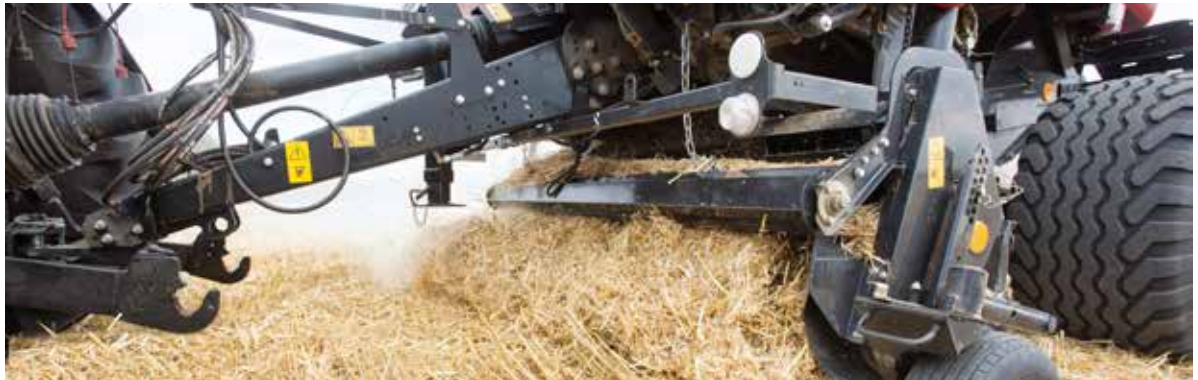
Swath delivery of short or long straw for perfectly formed bales
