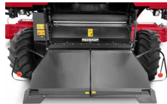
Xtra-Chopping system with independent spreadboards
