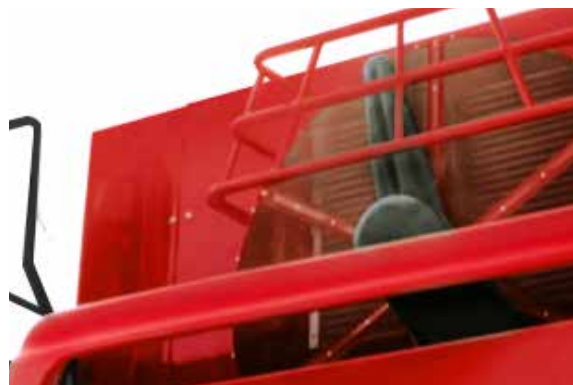
Fixed radiator grille for optimal dust clearing
