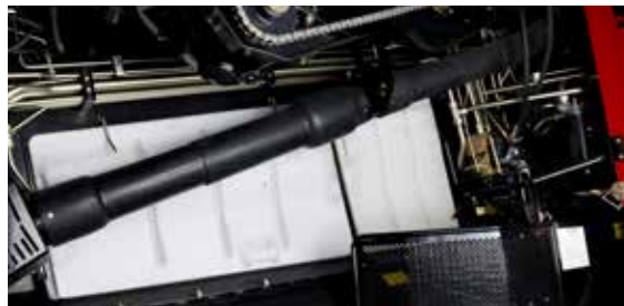
Power Plus drive transfers high power to the feed elevator and header. Simple, low-maintenance design
