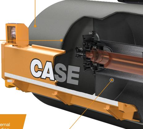
The centrifugal force is generated by an internal eccentric shaft and a rotating mass: depending on the direction of rotation, the rotating mass is in phase with the eccentric shaft for a maximum centrifugal force or in the opposite position, for a minimum centrifugal force.
