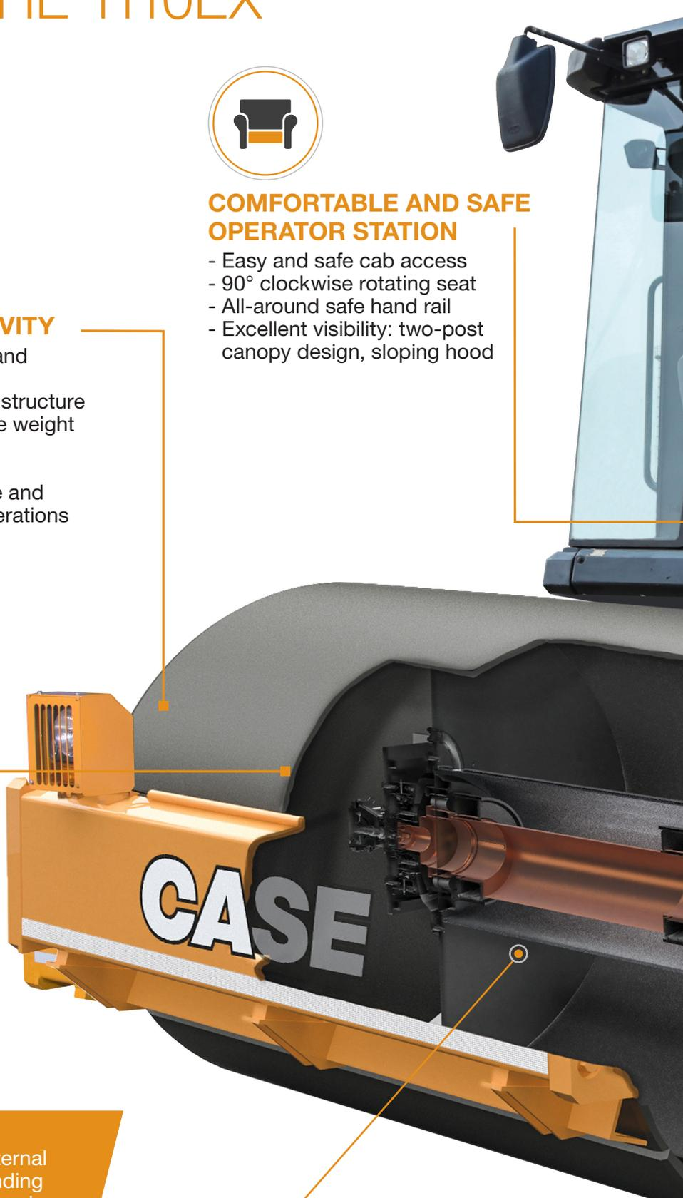
The centrifugal force is generated by an internal eccentric shaft and a rotating mass: depending on the direction of rotation, the rotating mass is in phase with the eccentric shaft for a maximum centrifugal force or in the opposite position, for a minimum centrifugal force.
