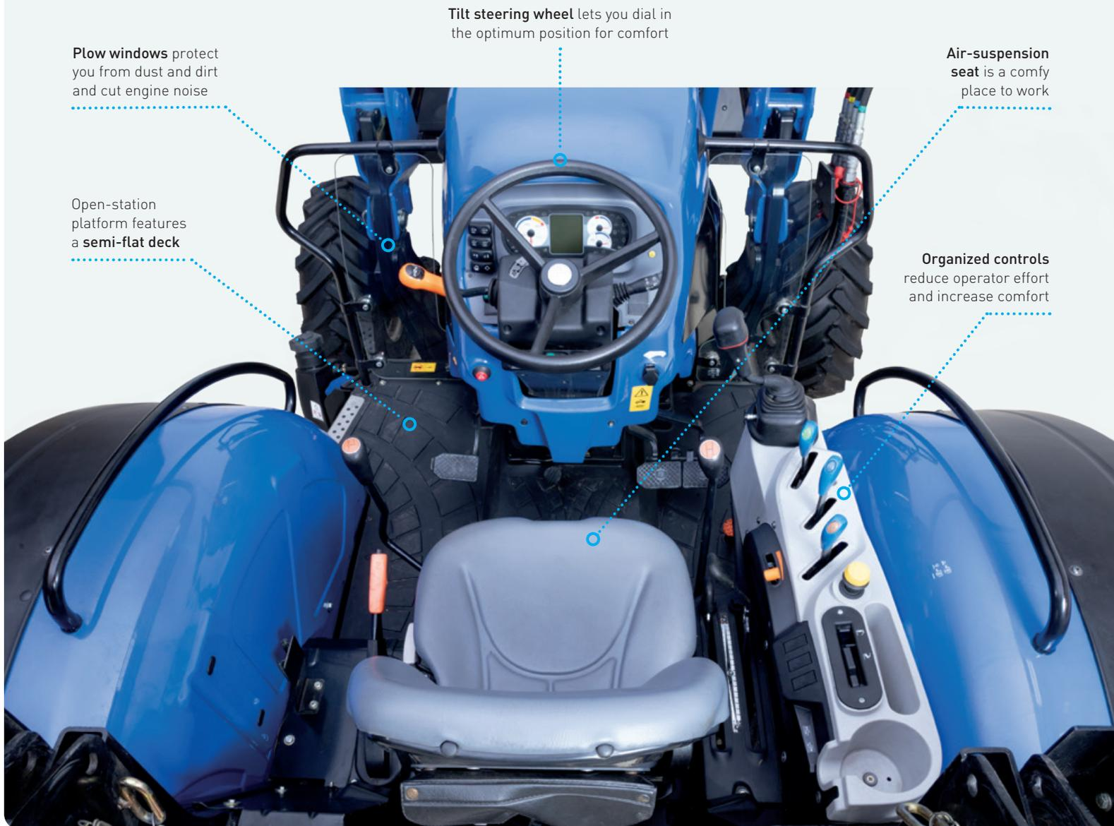
**Plow windows** protect you from dust and dirt and cut engine noise
