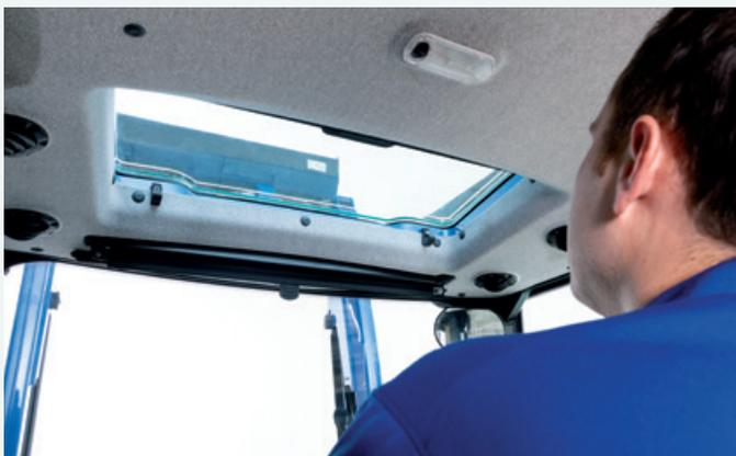
Optional **high-visibility panel** on all WORKMASTER™ cab models provides greater visibility, especially when working with a loader.
