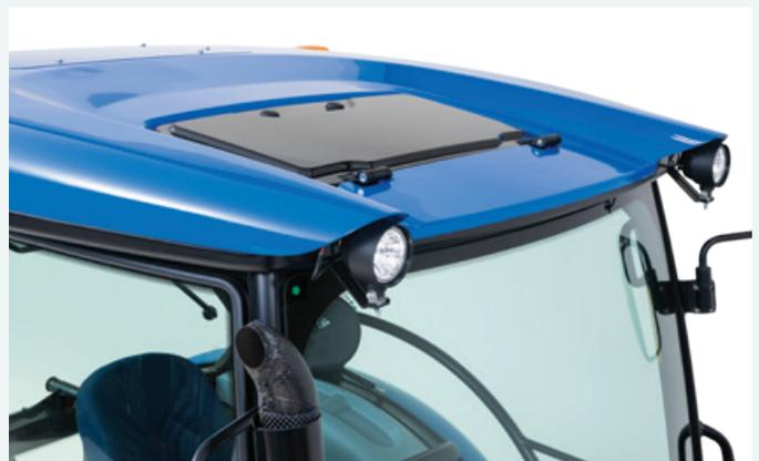
**HVAC system** features six roof vents and a blacked-out roof hatch that opens for ventilation.
