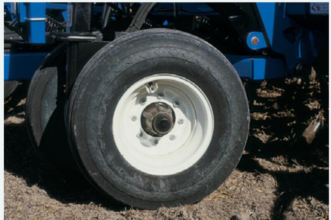
Dual walking casters provide optimum flotation.
