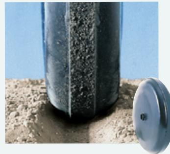
4-1/2 inch steel press wheels spread the packing pressure over a wider area for use when spreading seed or for wide double-shoot applications. The soil profile is the flattest of the steel wheels.
