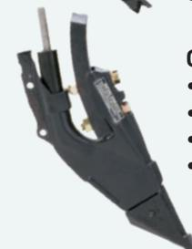
For paired row banding and side banding, New Holland Stealth openers have rubber grommets in them to insulate the cast opener from the cold NH<sub>3</sub> gas or liquid. This reduces the amount of freezing of the opener, which then reduces build up of frost and mud.
