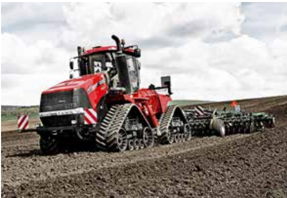
Magnum Rowtrac follows the same concept as Quadtrac with four points of contact to the ground.
