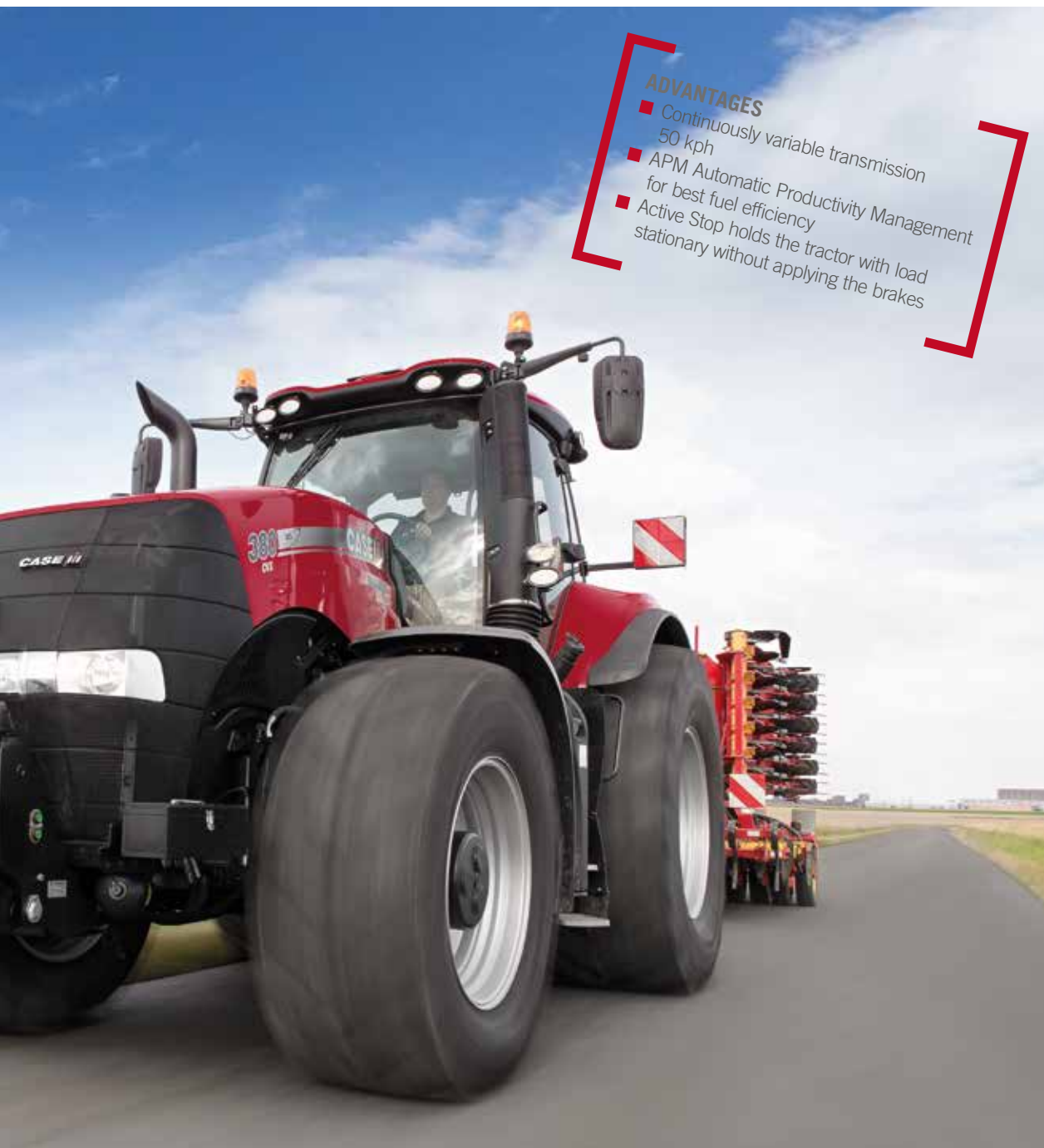
CVX transmission – stepless drive between 0-50 kph
