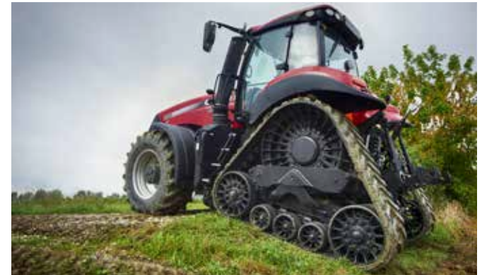
Wheels and tracks keeps in contact with the ground for maximum traction.
