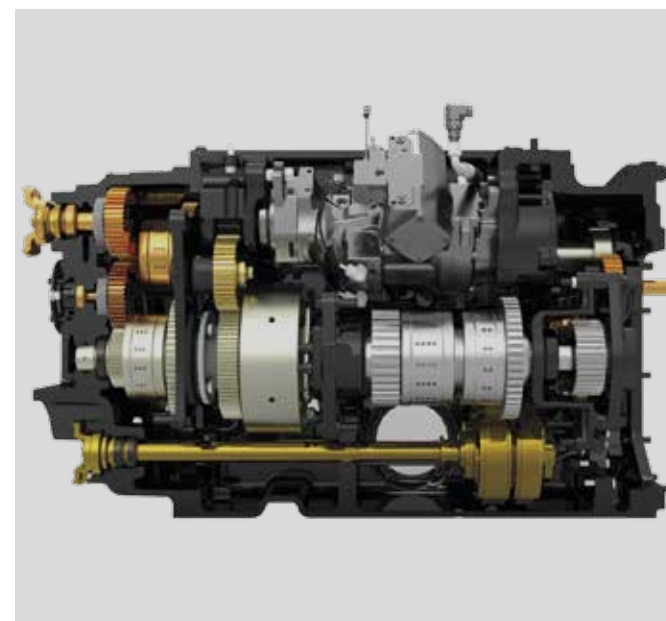
CVX transmission – stepless drive between 0-50 kph
