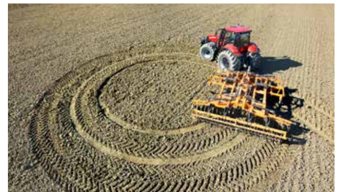
Unbeatable Turning Radius of 4.8 m.
