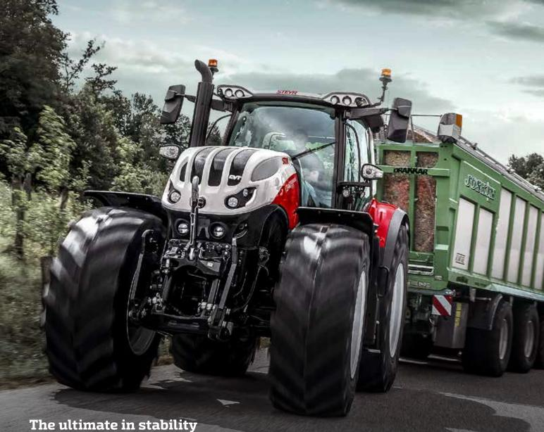
The TERRUS CVT series offers the most complete braking system on the market with S-BRAKE trailer braking systems. All the models are equipped with wet dual disc brakes (4 disc brakes on the rear axle). The more wear-resistant HD brake disc offers a longer service life, especially win heavy transport. Also, with an excellent power-to-weight ratio and a high maximum permissible weight, TERRUS CVT tractors are strong in the field and on the road.
