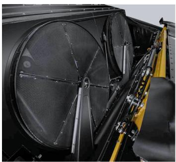
The CR10 features two cooling fans, with three on the CR11. Brushes on each rotary dust screen continuously clean the mesh in dusty conditions. All exhaust manifold/turbo/after-treatment components are fully insulated to reduce surface temperature of hot components. For maintenance, the cooling package is easily accessed by moving the rotor screens into the service position.
