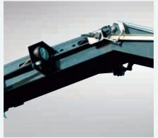
Six working lights have been placed in key working areas, including the spout, service deck and on the bumper to enhance foraging accuracy when working in low light conditions.
