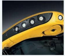
The FR lighting package offers up to 20 work lights including 17 LED lights. 11 LED lights have been precision placed in the roof to ensure the perfect spread of light.
