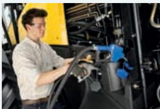
The fuel and 200 litre AdBlue tanks are conveniently located next to each other to facilitate simultaneous filling.
