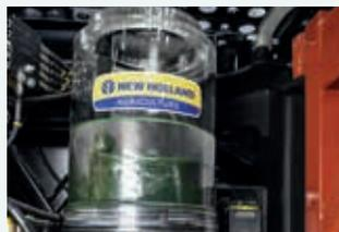
The centralised automatic greasing system is easy to access.
