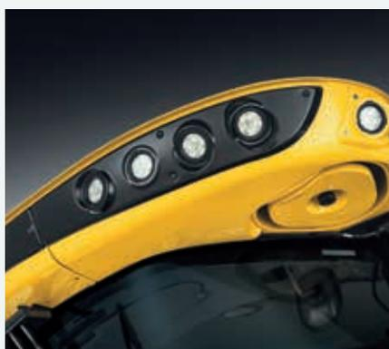
The FR lighting package offers up to 20 work lights including 17 LED lights. 11 LED lights have been precision placed in the roof to ensure the perfect spread of light.
