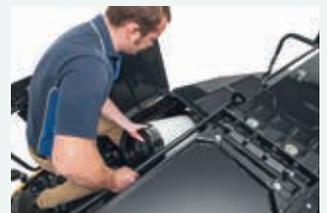
Convenient access to engine air filter.
