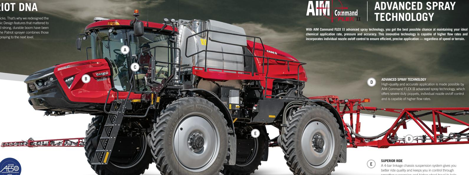
A 4-bar linkage chassis suspension system gives you better ride quality and keeps you in control through smoother suspension and higher wheel travel to help boost productivity.
