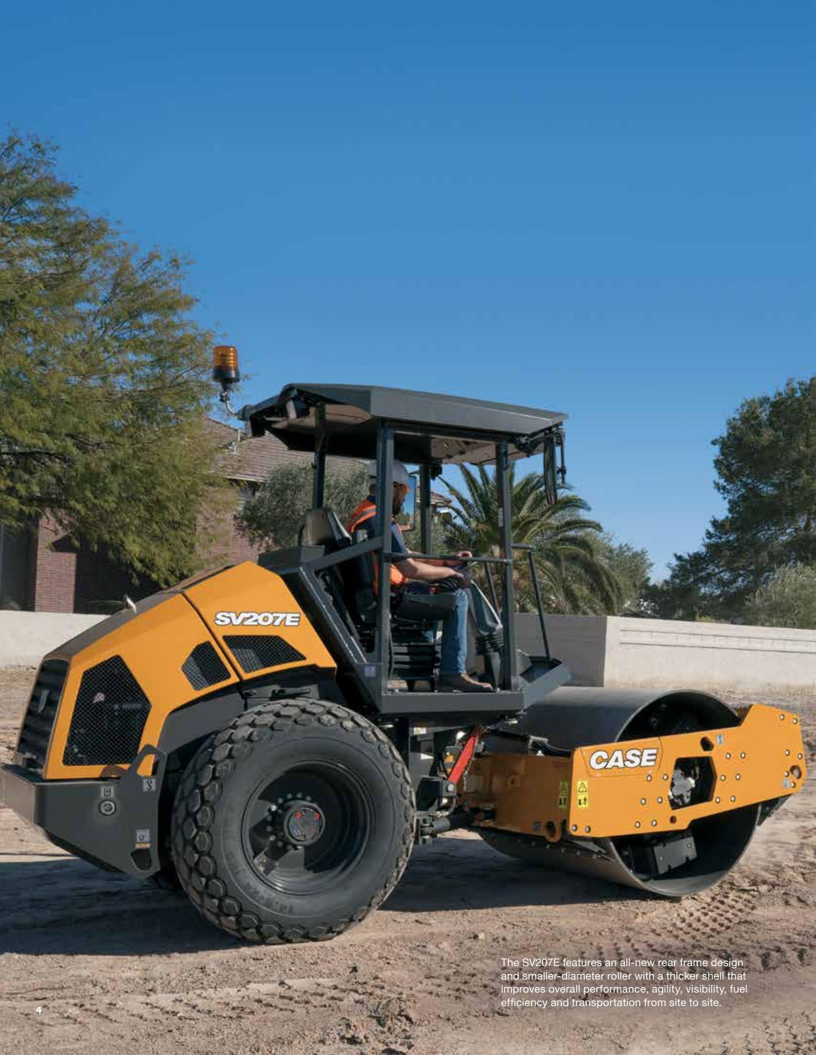
The SV207E features an all-new rear frame design and smaller-diameter roller with a thicker shell that improves overall performance, agility, visibility, fuel efficiency and transportation from site to site.
