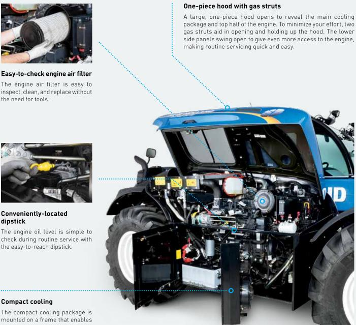
mounted on a frame that enables the radiators to both swing out and tilt for easy cleaning.
